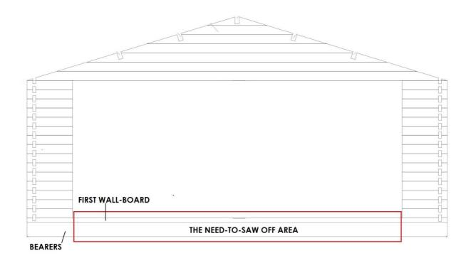
Assemble the garage door frame. Use screws:
