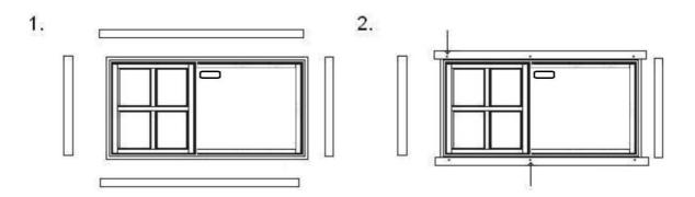
Screw the support trims in to the door frame and insert door frame in to its space from the outside of the structure. Then fix the rest of the support trims from inside the garage:
