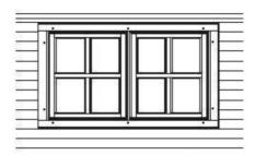
Now screw the rest four support trims in to the window frame from the other side.
