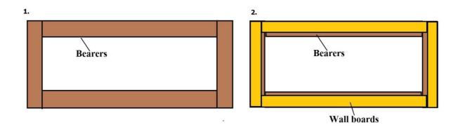
The wall-boards must be placed so that the ends interlock. Now screw the first row of wall-boards into the bearers. All the following rows of placed wall-boards should interlock not only at the ends, but along their length as well. Please screw each new row of wall-boards into the former row to ensure a solid structure.
